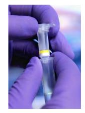
Silica Spin Column A silica spin column is used to purify the DNA
